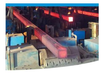
The structures on which the Deburring systems are installed are made with welded steel structures having characteristics suitable to operate in harsh environments such as those of the meltshops, and are designed with pneumatic handling systems.
